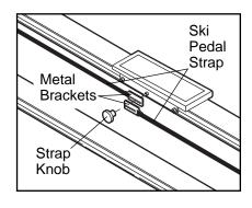
the metal brackets so that the ends of the strap are closer together. Slide the metal brackets back onto the ski pedal. Tighten the strap knob onto the ski pedal, making sure that the metal brackets remain parallel to each other as you tighten the knob.
